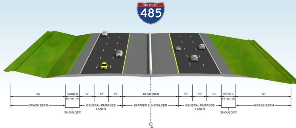
EXISTING TYPICAL SECTION (I-77 TO JOHNSTON ROAD)
