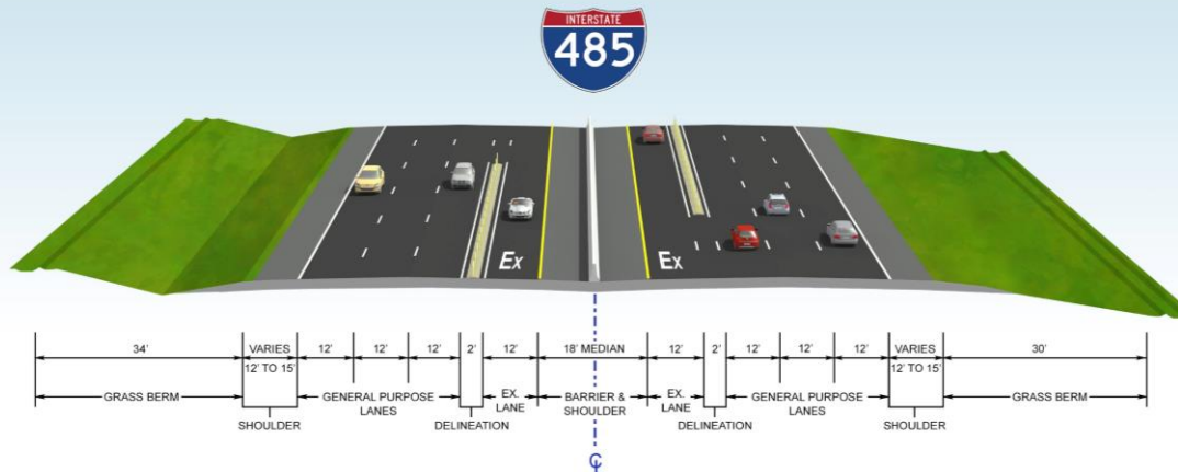
PROPOSED TYPICAL SECTION (I-77 TO JOHNSTON ROAD)
