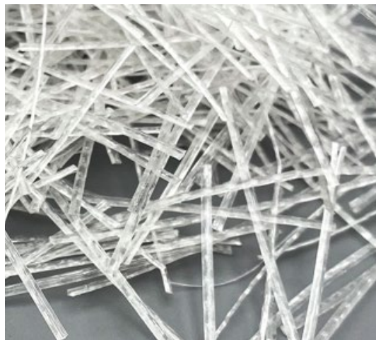
Image of Nycon XL-200 fibers (left) from Nylon's product catalog and a 50x magnified fiber sample (right) from Nycon's lab test report.
