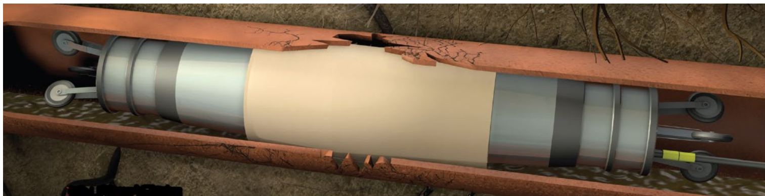
Illustration of a damaged pipe being repaired by the HammerHead® Point Repair Kit from HammerHead's product brochure.
