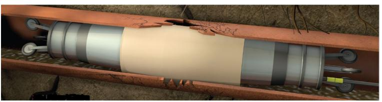
Illustration of a damaged pipe being repaired by the HammerHead® Point Repair Kit from HammerHead's product brochure.
