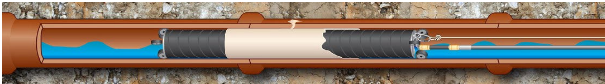
Images of a PipePatch® repair illustration, a damaged underground concrete pipe, and the concrete pipe repaired using PipePatch® from Source One Environmental's website.
