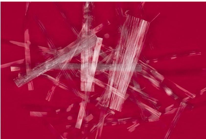
FiberForce 750, by FullForce Solutions, is a blend of synthetic macrofibers used for improving tensile strength, durability, reducing plastic shrinkage and settlement cracking in concrete. The fibers are blended into ready-mix drums filled with concrete and can be used in the construction of concrete slabs, precast structures, bridge decks, and concrete paving. FiberForce 750 is Approved for use on the APL as NP23-9381.
