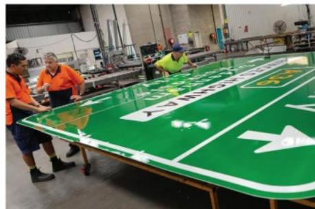
ORALITE® 9900 Brilliant Grade Premium is a highly reflective, weatherproof, self-adhesive reflective sheeting product with excellent corrosion and solvent resistance used for permanent outdoor signing. It consists of sealed cells of air backed microprisms using total internal reflection and is available in a full range of colors. ORALITE® 9900 is manufactured by ORAFOL Americas, Inc. and is Approved on the APL as NP23-9239.
