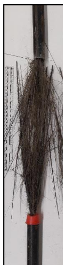
Various diameter samples of white BFRP rebar (left); sample of black BFRP rebar after tested to its tensile strength failure limit (right) – images from Pultrall website (left); and from Pultrall testing report (right)
