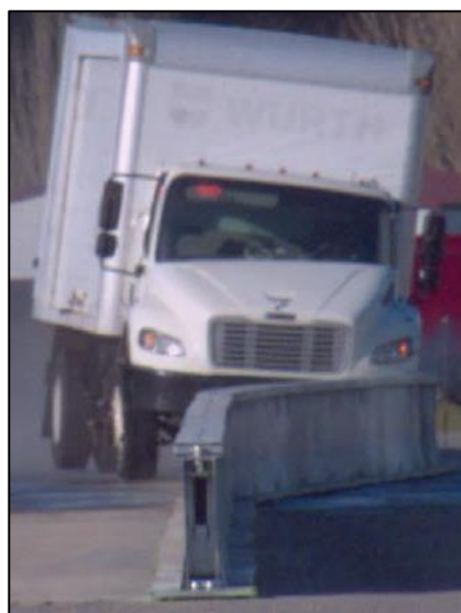
Example of a box truck colliding with, and being safely deflected by the HighwayGuard ™ system – image from HighwayGuard website
