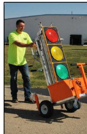
Worker collapsing the JTI Sentinel™ mounted on a moveable hand cart – image from JTI Sentinel™ brochure
