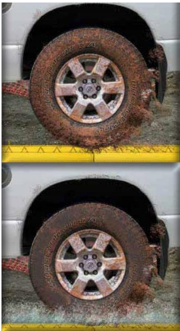
Before & after image of small truck tire using Rumble Rack – image from ACF Environmental Brochure
