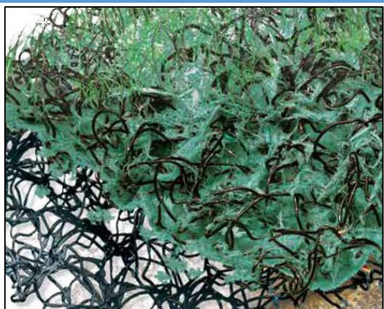
Futerra TRM (black fibers) with Flexterra HP-FGM (green fibers) hydraulically applied and grass growing at top of image – image from GreenArmor 7020 brochure
