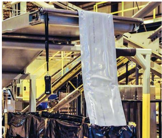
Example of pipe-liner coming off manufacturing line – image from Reline America website
