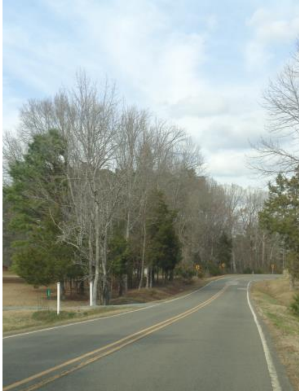
4" Paint SR 1136 (Tally Ho) Granville Co. Install Date Pre-2013 (Estimated) Photo Taken March 2018 (Retro Data: CL 62/EL 85)
