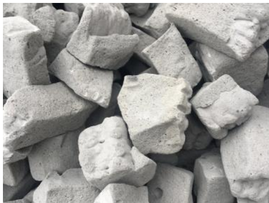
Close-up image of FGA G15 – image from Aero Aggregates' website
