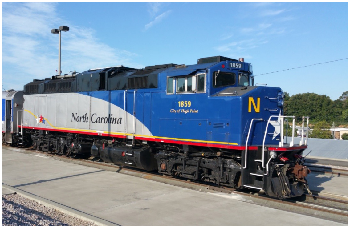
NCDOT locomotive 1859 fitted with the Blended After-Treatment System (BATS) (Photo: Rail Propulsion Systems)
