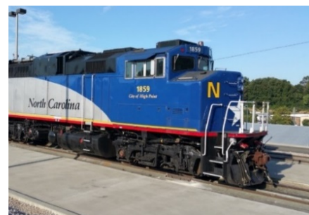
NC 1859, the first locomotive fitted with BATS and certified by the EPA
