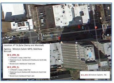
Figure 7. Example site diagram; aerial image shows location of equipment and sensors, labeled facilities, and is oriented north.
